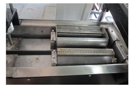
c.Open a tin furnace for heating temperature
