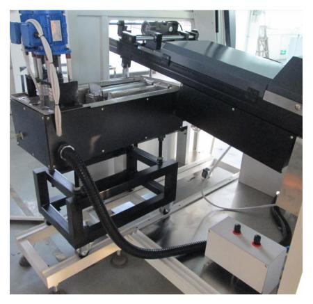
a, the tin stove frame is installed in the position of tin stove in and out .
