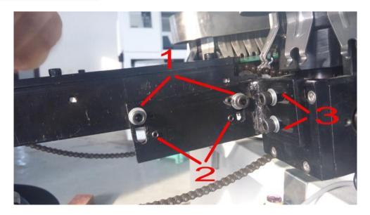
Note: 1.Conveyor guide high and low level adjustment
